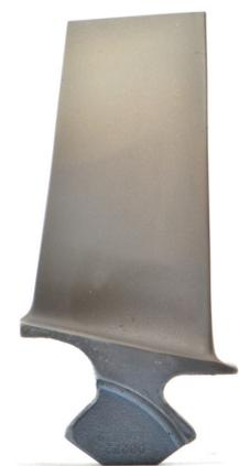
**Figure 1.** High-pressure compressor (HPC) blade.
